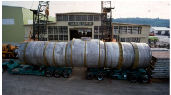
Heating element of a vapor recompression evaporator being carefully prepared for special shipment.
